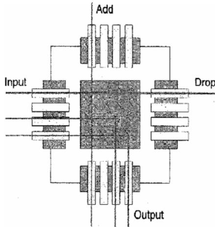
Fig. 1. MEMS switch [1].
